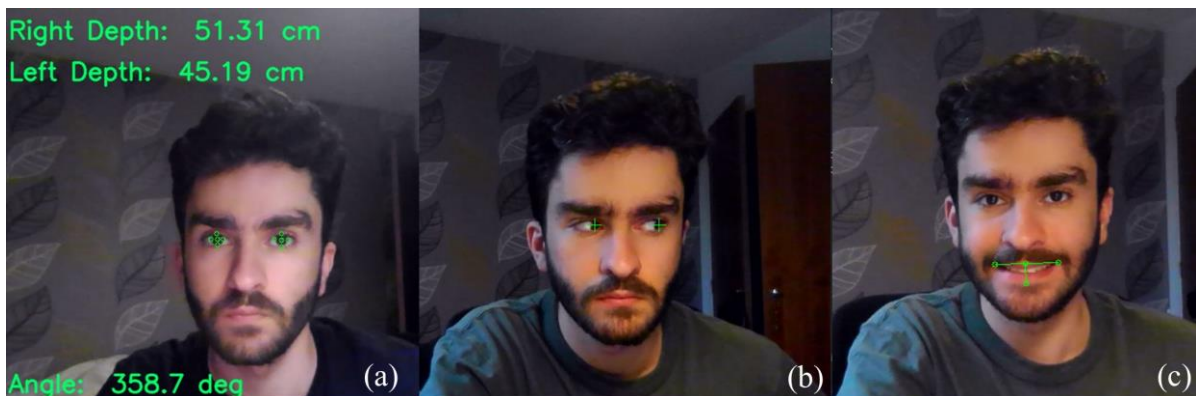
Figure 2: Simplified framework using (a) Depth calibration, (b) eye tracking, and (c) mouth tracking.
