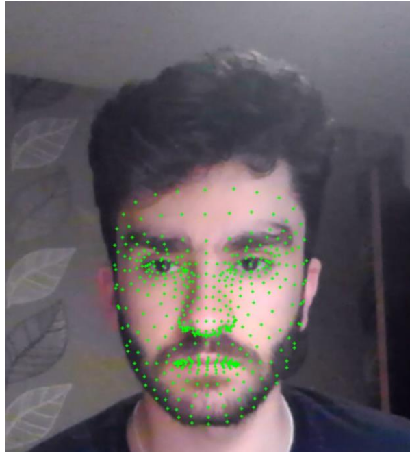
Figure 1: 468 facial landmarks estimated in 3D using a basic camera.
